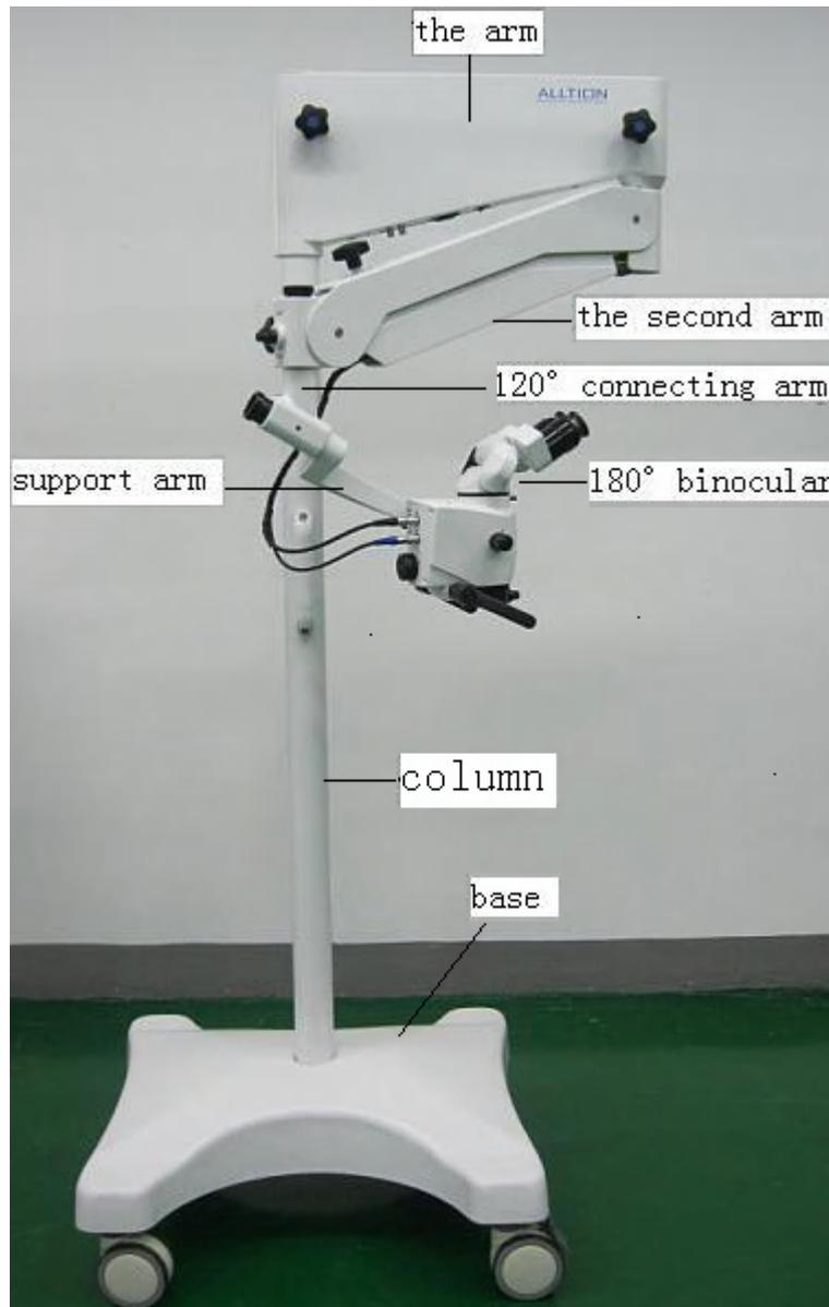
Fig 4 Assembly drawing of Microscope
